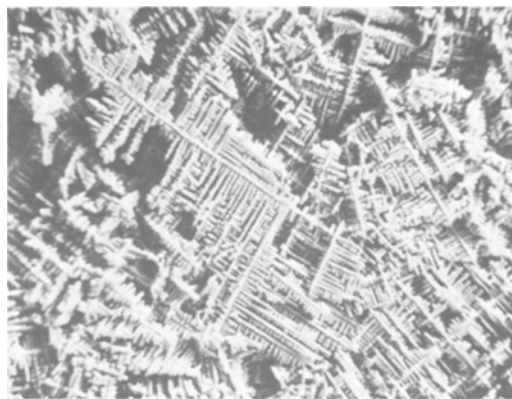
Figure 3 Cu-20 wt% Nb alloy cast from a ThO_2 crucible and etched for 3 min, \times 364 .
